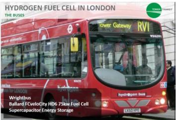
David Yorke of Tower Transit explained that their fuel cell buses have been in regular service in London for many years. As well as the Wright Bus, they operate fuel cell buses from Van Hool. They are planning to scale up operations with fuel cell buses to be a world leading operator in this field.
